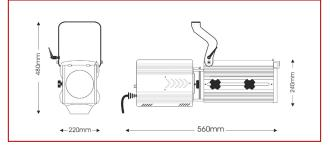
Stylish, compact and extremely high efficiency very wide angle LED zoom profile featuring a 380W RGBW COB power source and double-condenser optics. Alba is DMX/RDM controllable for 16 bit dimming.
