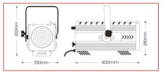
A high efficiency led module featuring a 380W RGBW COB power source harnessed in the high-specification optics of LDR fresnel spotlights.
