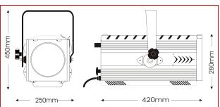
A high efficiency led module featuring a 380W tunable white COB power source harnessed in the high-specification optics of LDR pebble-convex spotlights.
