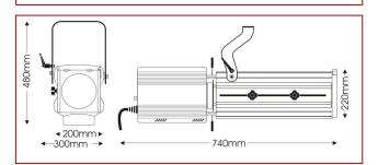
Stylish, compact and extremely high efficiency wide angle LED zoom profile featuring a white 150W led COB power source and double-condenser optics. Recently introduced specifications include RDM control for 16 bit dimming, 3 choices on fan speed control and increased light output.
