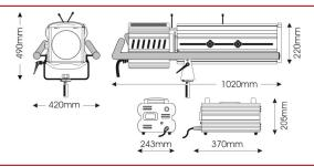
The Canto® 1500msr FF is an, efficient, lightweight and extremely powerful followspot, ideal for all medium to long-throw applications. The MSR filling of the lamp guarantees pure, white light, whereas the short arc provides high beam intensity for professional entertainment lighting.
