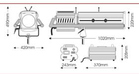
The Canto® 2000msr FF is an, efficient, lightweight and extremely powerful followspot, ideal for all medium to long-throw applications. The MSR filling of the lamp guarantees pure, white light, whereas the short arc provides high beam intensity for professional entertainment lighting.
