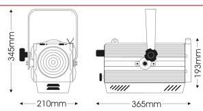
Stylish, compact and high efficiency RGBW led power source, fresnel luminaire featuring 120mm diameter Fresnel lens and DMX/RDM controllable for 16 bit dimming and infinite colour beams.
