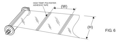
Use High Temperature Transparent Polyester adhesive tape (e.g. 3M #853) to join the colour filters side by side (FIG.6). Make sure that there is a good adhesion by pressing firmly on the tape against the filters. Join the first and the last color filter to the rollers. You can use the reference line marked on the roller for alignment. Please note that the tape should be taped on the side facing you on the rollers.
