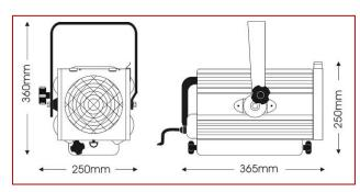
Quality 1/1200W fresnel spotlight including screw focus, variable spread, soft-edged beam, front hinging lamp tray, tilt lock and double-microswitch interlock for safe lamp replacement.
