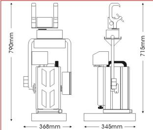
The perfect combination of the extremely popular Nota pc1200 pebble-convex luminaire, the totally reliable Xpress 19 colour scroller and a remote control yoke. Nota pc1200 Moving is an extremely high-specification product featuring pan, tilt and zoom remote control, plus a vast choice of options for the professionals.
