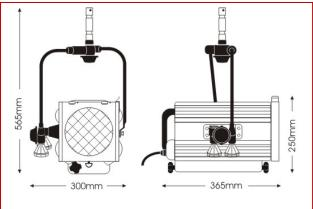
Quality 1/1200W pebble-convex spotlight fitted with a pole-operated stirrup to control pan and tilt movement. It's ideal for all those applications where the luminaires are difficult to access and whose position needs to be changed frequently. It includes screw focus variable spread softedged beam, front hinging lamp tray, adjustable lamp-base and double-microswitch interlock for safe lamp replacement.
