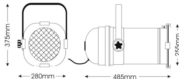
This 1000W Par 64 range offers a choice of finish – black or natural polished aluminium – with either a regular or short length tube. A model with fitted rear lamp rotator is also available. A colour frame and wiring kit is included as standard.
