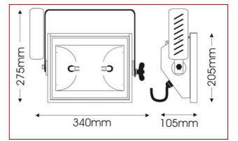
Stylish and high specification 70W symmetrical discharge floodlight, ideal for usage in all those architectural, display and retail areas applications where a powerful yet low consumption and long lasting beam of light is required.
