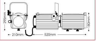
Ideal for closer-range highlighting, this 20°-40° profile spotlight uses a compact 70W discharge lamp combined with a double-condenser optical system to project a crisp flat beam particularly suited for projecting patterns or advertising logos in architectural and display applications. The cool beam design enables a wide range of metal, dichroic or acetate gobos and slides to be used.
