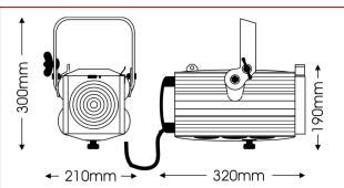
Ideal for display lighting and theatrical-style illumination of architectural spaces, the Soffio Fresnel produces a bright soft-edged beam, variable from 7° to 63°, shaped using an optional 4-leaf barndoor accessory.
