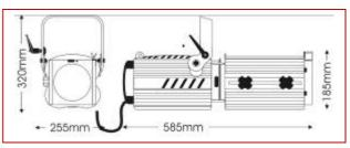
The wider-angle Suono D profile spotlight has a variable zoom focus from 20° to 40°, making it suitable for short-throw applications. The 250W MSD lamp produces a high-power 'daylight' beam which is popular for display, retail and architectural lighting.
