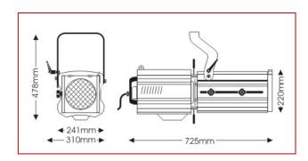
For closer projection in larger venues, this wide-angle 18° - 36° 2000W spotlight incorporates a zoom focus double condenser optical system, rotating gate, a cranked fork and a double microswitch interlock for safe lamp replacement.
