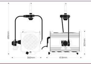
Compact, lightweight and powerful 2/2.5KW fresnel spotlight. It features an extremely wide beam angle and includes a height adjustable, robust G22 lamp-base, screw focus, improved tilt lock and double-microswitch interlock for safe lamp replacement.
