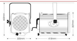
The best performing Fresnel 1000/1200W luminaire on the market, the Nota F1200 XL features a 200mm high quality borosilicate lens, which enhances the light output for throws up to 25m of a perfectly smooth, soft-edged beam.
