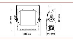
180 watt LED RGBW asymmetrical floodlight ideal for cyclorama-type lighting in all applications.
