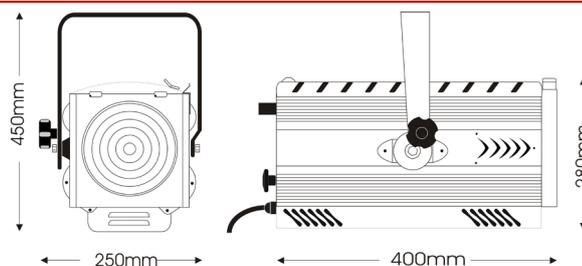
A high efficiency led module featuring a 380W tunable white COB power source harnessed in the high-specification optics of LDR fresnel spotlights.
