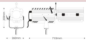
New, stylish, compact and high efficiency 120W RGBW led narrow-angle followspot featuring double-condenser optics and a PWM dimming power source. ASTRO 100 is DMX512 and RDM controllable for infinite colour beams but manual dimming from rear panel is also an option.
