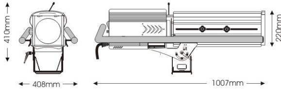
Stylish, compact and extremely high efficiency followspot featuring a 230W white LED power source, digital dimming, flicker free and constant colour temperature at any light intensity and producing a powerful and highly-defined beam of pure white light.
