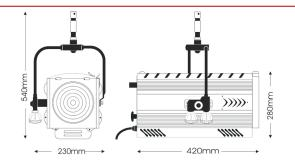
A high efficiency led module featuring a 380W RGBW COB power source harnessed in the high-specification optics of LDR fresnel spotlights and a PO stirrup for the control of pan and tilt movement.
