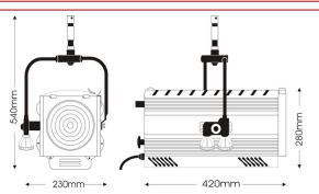
Stylish, compact and extremely high efficiency RGBW led power source Fresnel luminaire, DMX/RDM controllable for 16 bit dimming and infinite colour beams, fitted with a PO stirrup for the control of pan and tilt movement.
