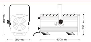
A high efficiency 150W led module featuring a PWM dimming power source harnessed in the high-specification optics of LDR fresnel spotlights. Recently introduced specifications include RDM control for 16 bit dimming, 3 choices on fan speed control and increased light output.
