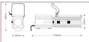
Stylish, compact and extremely high efficiency wide angle LED profile zoom featuring a 380W Tunable White COB power source and double-condenser optics. Alba is DMX/RDM controllable for 16 bit dimming.
