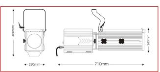
Stylish, compact and extremely high efficiency wide angle LED zoom profile featuring a 230W led COB power source and double-condenser optics. Alba is DMX/RDM controllable for 16 bit dimming.
