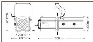
This wide-angle 1000/1200W profile spotlight includes high-specification double condenser optical system for clean, crisp gobo projection.
