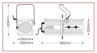
This extremely wide-angle 1000/1200W profile spotlight includes high-specification double condenser optical system for clean, crisp gobo projection.
