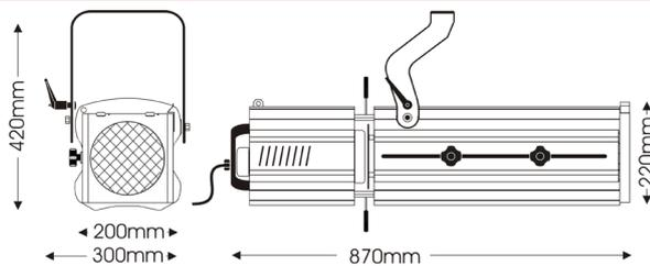
A high-specification 1000/1200W profile spotlight with advanced features including a double condenser optical system for extremely sharp gobo projection, rotating 4-shutter gate, 8° to 22° narrow-angle zoom focus, a double-microswitch interlock for safe lamp replacement, easy access for lens cleaning and a cranked fork. Ideal for front-of-house projection positions.
