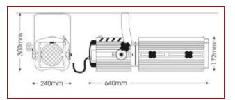
Compact and high-specification 500W/650W profile spotlight with a double-condenser zoom focus optical system to provide crisp projection of gobos and a brilliant flat beam between 10° and 28°.
