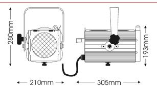
Simple yet high-quality 650W PC spotlight featuring a slide-focus variable-spread beam to offer more definition than the softer Fresnel beam.
