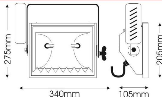
Stylish and high specification 150W asymmetrical discharge floodlight, ideal for usage in all those architectural, display and retail areas applications where a powerful yet low consumption and long lasting beam of light is required.
