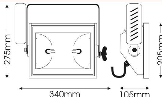
Stylish and high specification 150W symmetrical discharge floodlight, ideal for usage in all those architectural, display and retail areas applications where a powerful yet low consumption and long lasting beam of light is required.
